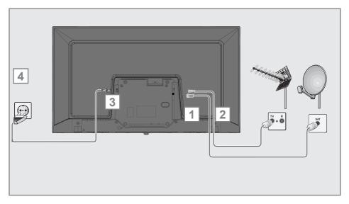
To receive digital satellite channels (DVB-S), connect the satellite antenna cable to the antenna socket SATELLITE on the television set;
